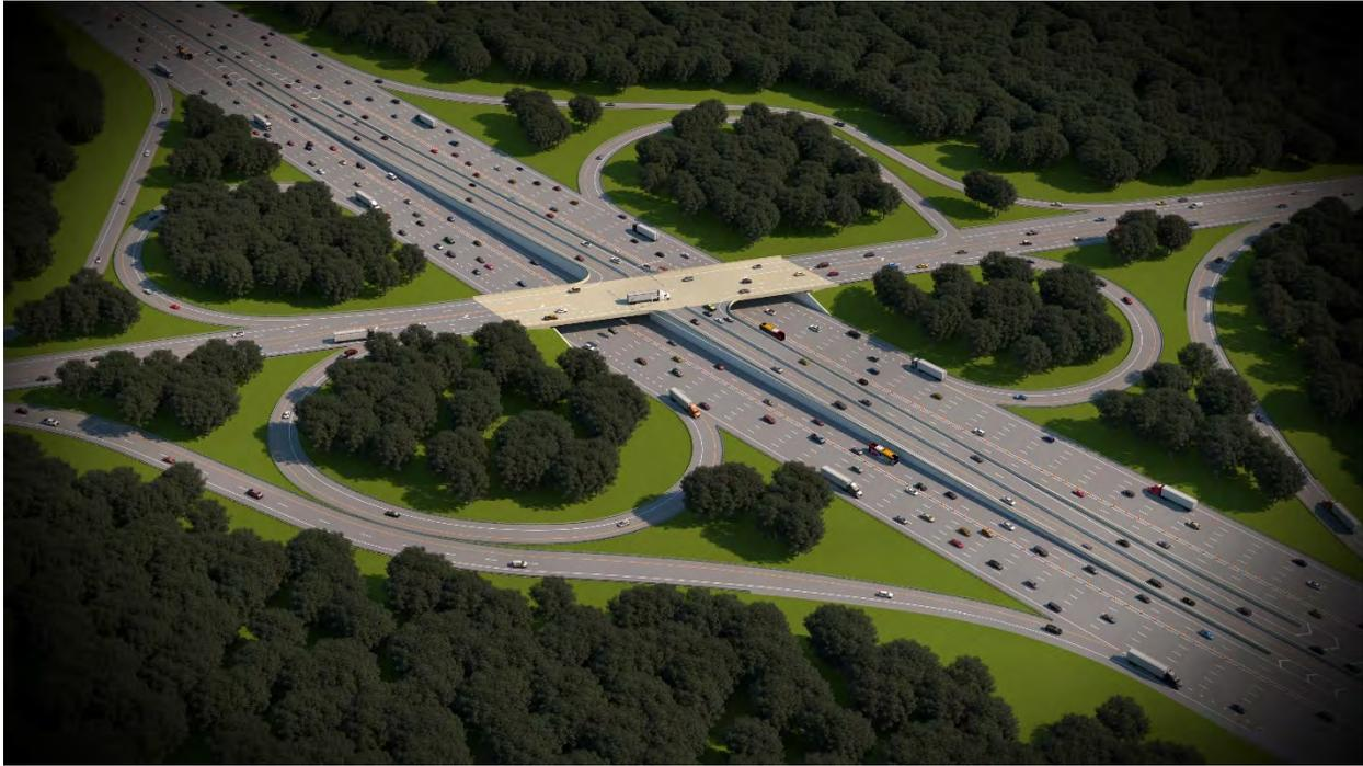
Figure 5-8: Example At-Grade Access Slip Ramp Configuration
